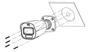
(5) Bracket adjustment. Before adjustment, preview the image of the camera on a monitor and then loosen the fixed ring to adjust the view angle of the camera.
