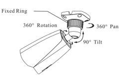
(6) Tighten the fixed ring to complete the installation.
