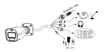
\* 1 It is recommended to install the security cap for outdoor installation.
