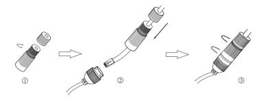
1 Loosen the nut from the main element.
