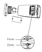
**(6)** Install the cover back to the camera and fix it firmly with the screws. (Note that the cover should not be installed unevenly.)
