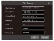
⑤ Checkmark the device you want to add and then click "Add" button. The NVR will automatically refresh the cameras and return to "Edit Camera" interface. "Online" status means connecting the device successfully and you will see the live image. You may select the added device and click ■ button to modify channel, IP address, ect.
