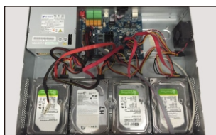
⑤ Connect the power and data cables.
