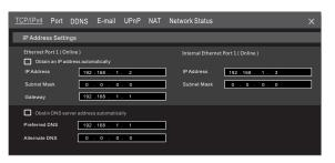
④ Go to Start → Settings → Camera → Add Camera. The NVR will automatically refresh the cameras searched. The IPC which supports the Onvif protocol may be added manually. If the IPC searched is not in the same local network as the NVR, you should select the device and click ■ to modify the IP address.
