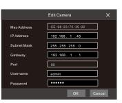
⑤ Checkmark the device you want to add and then click "Add" button. The NVR will automatically refresh the cameras and return to "Edit Camera" interface. "Online" status means connecting the device successfully and you will see the live image. You may select the added device and click ■ button to modify channel, IP address, ect.
