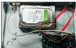
④ Connect the power and data cables.
