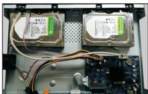
③ Put the HDDs onto the bottom of the machine.
