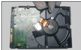
② Screw the screws into the holes of the HDD but not tighten them.
