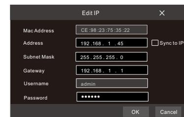
⑤ Checkmark the device you want to add and then click “Add” button. The DVR will automatically refresh the cameras and return to “Edit Camera” interface. “Online” status means connecting the device successfully and you will see the live image. You may select the added device and click button to modify channel, IP address, ect.
