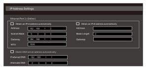
④ Go to Start → Settings → Camera → Add Camera. The DVR will automatically refresh the cameras searched. The IPC which supports the Onvif protocol may be added manually. If the IPC searched is not in the same local network as the DVR, you should select the device and click to modify the IP address.
