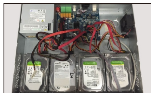
⑤ Connect the power and data cables.
