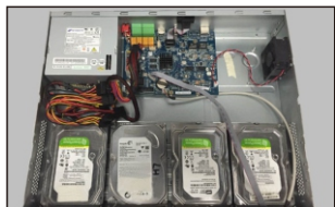
④ Install the other three HDDs according to above-mentioned method.
