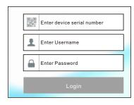
**Device Serial Number**: Click  $\blacksquare$  on the menu bar at the bottom of the live interface to check the serial number or go to Start  $\rightarrow$  Settings  $\rightarrow$  Network  $\rightarrow$  Network Status to check the serial number of the DVR).
