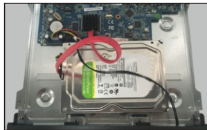
④ Connect the power and data cables.
